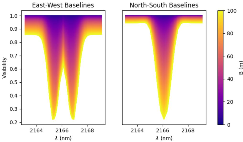
As expected, for a rotating disk (see Meilland et al. (2012) for more details), the visibility for the baselines along the major-axis show a W-shaped profile through the line, whereas the visibility along the minor-axis of the disk show a V-shaped profile.
