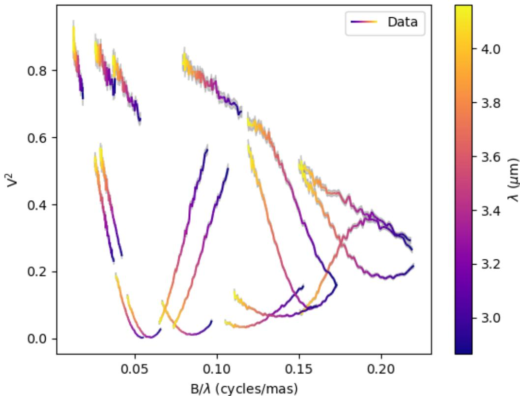
We can also plot the square visibility as the function of the wavelength while colouring the curves by the interferometer configurations (i.e., the list of all baselines within one file). Note that we can pass parameters to the error plots with the `kwargs_error` keyword.
