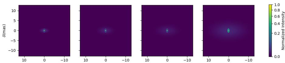
Although quite complex this models only have 9 free parameters. If we change the ellipse diameter and its position angle, the components will scale (except the Gaussian that fwhm is independent) and rotate.
