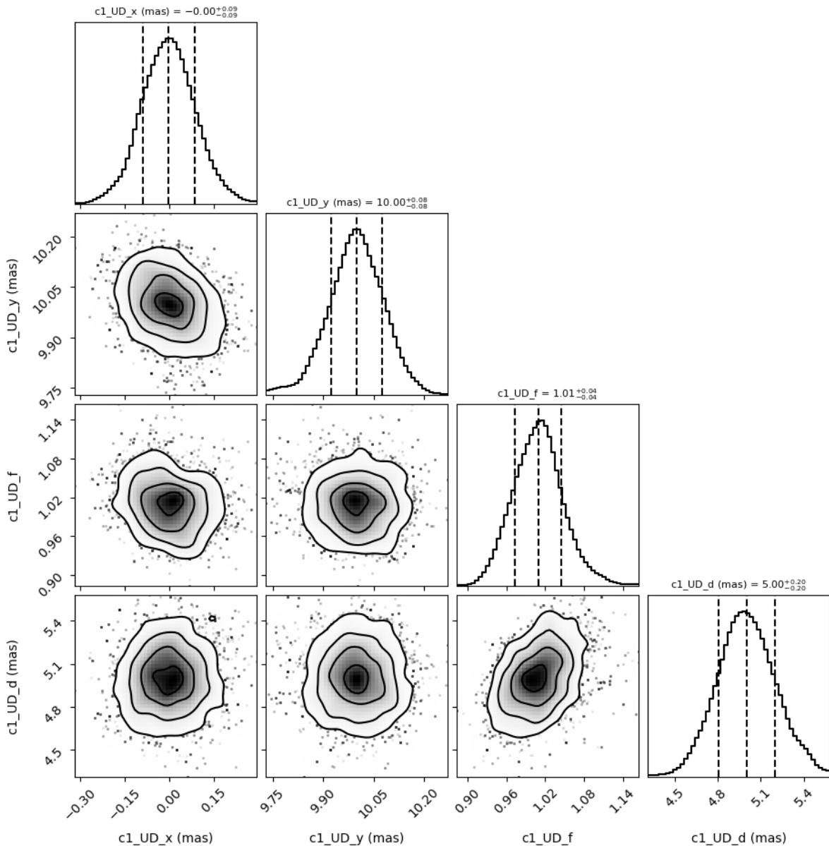
We now can retrieve the result of our fit. The `oimFitterEmcee` fitter can either return the "best", the "mean" or the "median" model. It also returns uncertainties estimated from the density distribution (see emcee's documentation for more details on the statistics).
